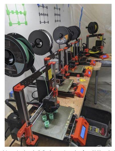
Courtesy photosA row of 3-D printers set up in a plastic-lined garage to produce face shields and splitters for ventilators.
