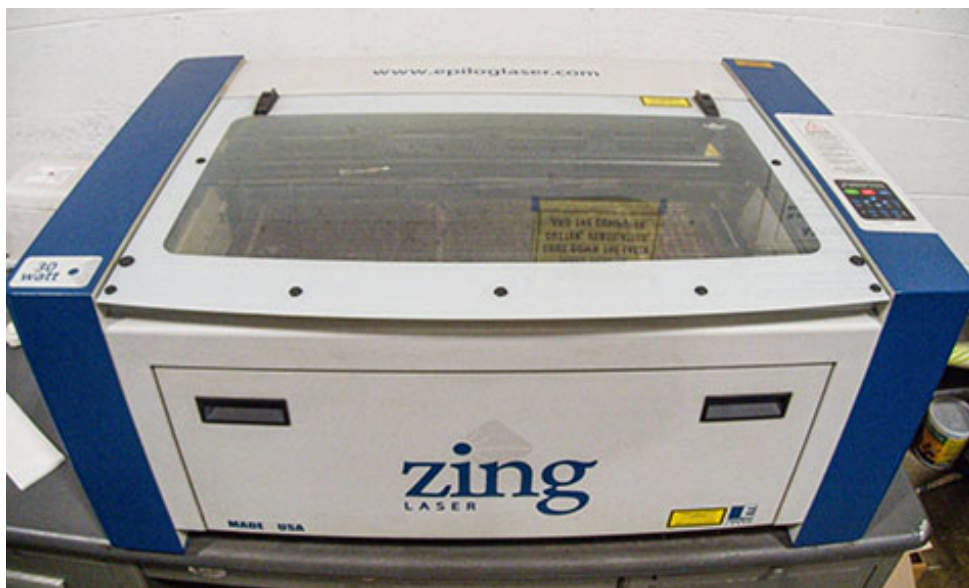
The Zing machine is a laser cutter that cuts the clear plastic of the mask. (Photo by Lipofskyphoto.com)
